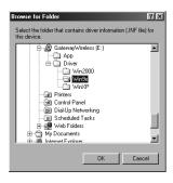
5 Navigate to the *Driver* folder located on the installation CD. For example, if you are installing drivers for Windows 98SE, click to highlight the Win9X folder located under the *Driver* folder on the installation CD.
